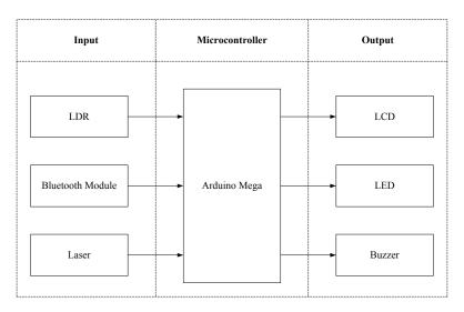
Figure 2: Block diagram of the prototype
